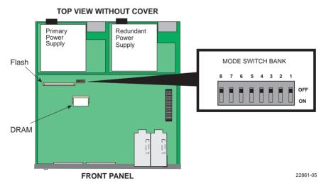
Figure C-2 Mode Switch Location/Component Layout
